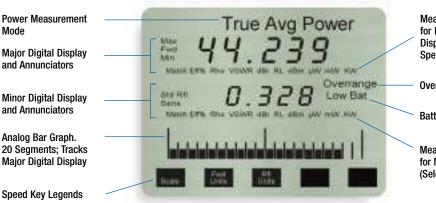
Measurement Units for Major Digital **Display (Select with** Speed Key)
